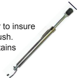
2. Holding the instrument firmly, press slowly against a given door at a point approximately handle-high, and 30 inches toward the handle from the door's hinges.
